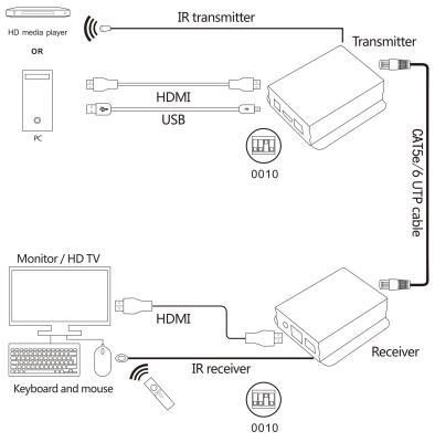
(Set IP address of the transmitter and receivers to the same)
