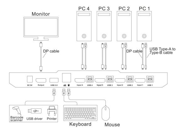
**Note:** The mouse and keyboard can implement hotkey functions when connected to a dedicated mouse and keyboard port.
